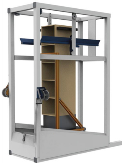
Fig. 6 The Impact Tester, used to evaluate packages in conditions similar to those on a pallet in a braking truck.
